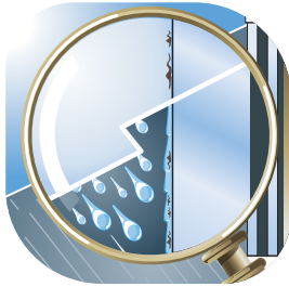
The photocatalytic action of Pilkington Activ™ glass (upper) gradually breaks down and loosens organic dirt, while the hydrophilic surface (lower) causes rain to sheet on the glass, leaving a clean exterior with minimal spotting or streaking.
